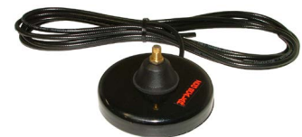
SKU: MGB-OB Magnetic OB-2 Base, steel with polished black powder coat finish, 10.5 cm diameter, heavy duty magnet, PVC matted pad on bottom, 4.7 metres RG58 low loss stranded cable side exits, no connector
